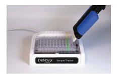
Sample Tracker Software-controlled LEDs illuminate the correct sample column
