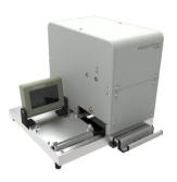
The Ultraseal™ ePRO-MINI is designed for automated workflow systems requiring a sealing step for a medium rate of plate usage. The design uses individual sheets loaded in a proprietary frame format, eliminating the need for large rolls of seals used by high throughput sealing instruments.
