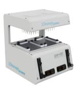
The nitrogen drydown process is ideal for lower boiling point organic solvents such as methanol, dichloromethane, hexane and acetonitrile. The robust design of the Ultravap® Gemini evaporator brings together for the first time in our range two individually temperature-regulated evaporation positions with a wide choice of head styles and configurations. This means you can dry down a 96-well deep well plate at the same time as 48 HPLC vials. This breakthrough in productivity will
