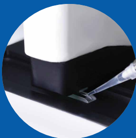
Load Cell Suspension into Sample Chamber
